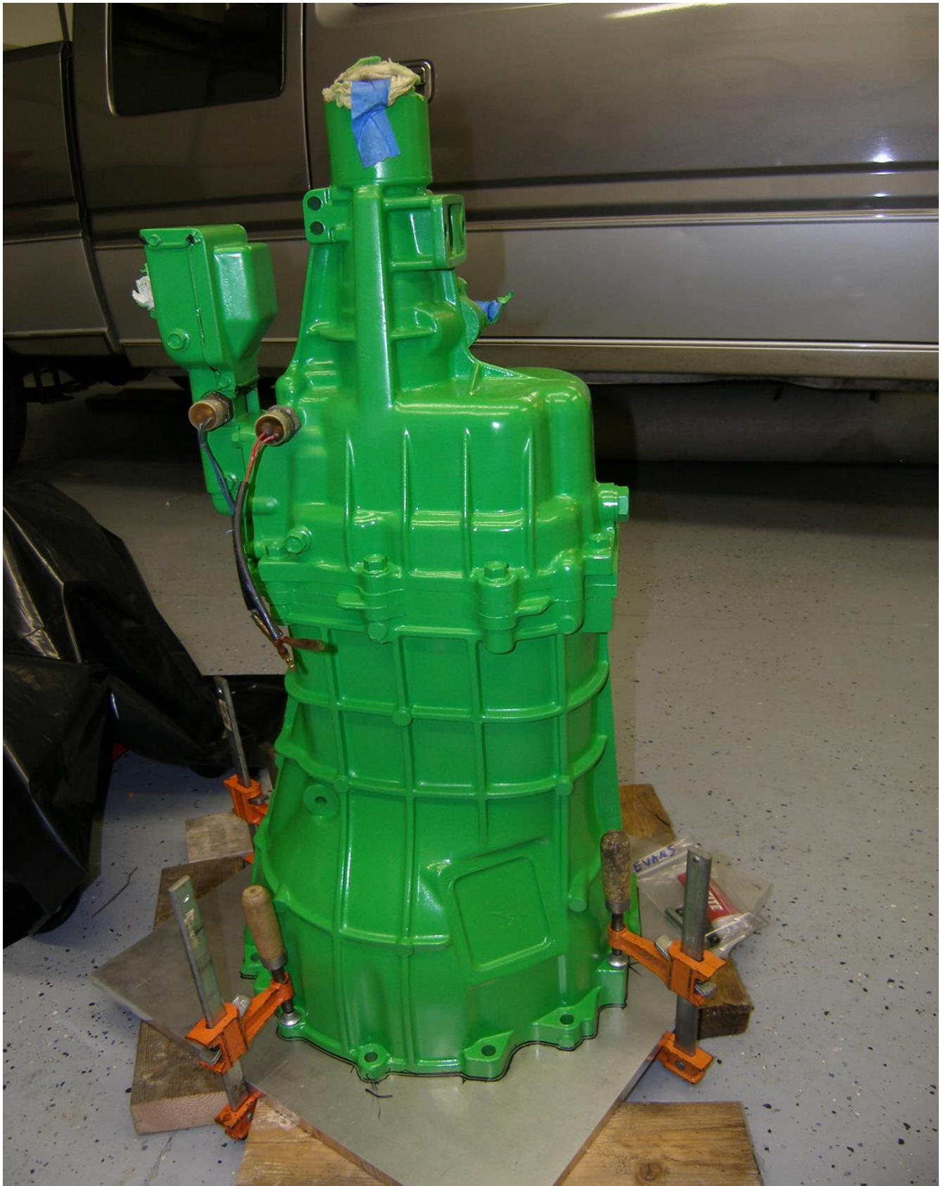
Figure 5 – 4 The clutch housing sitting on top of the transmission-motor transition plate.
