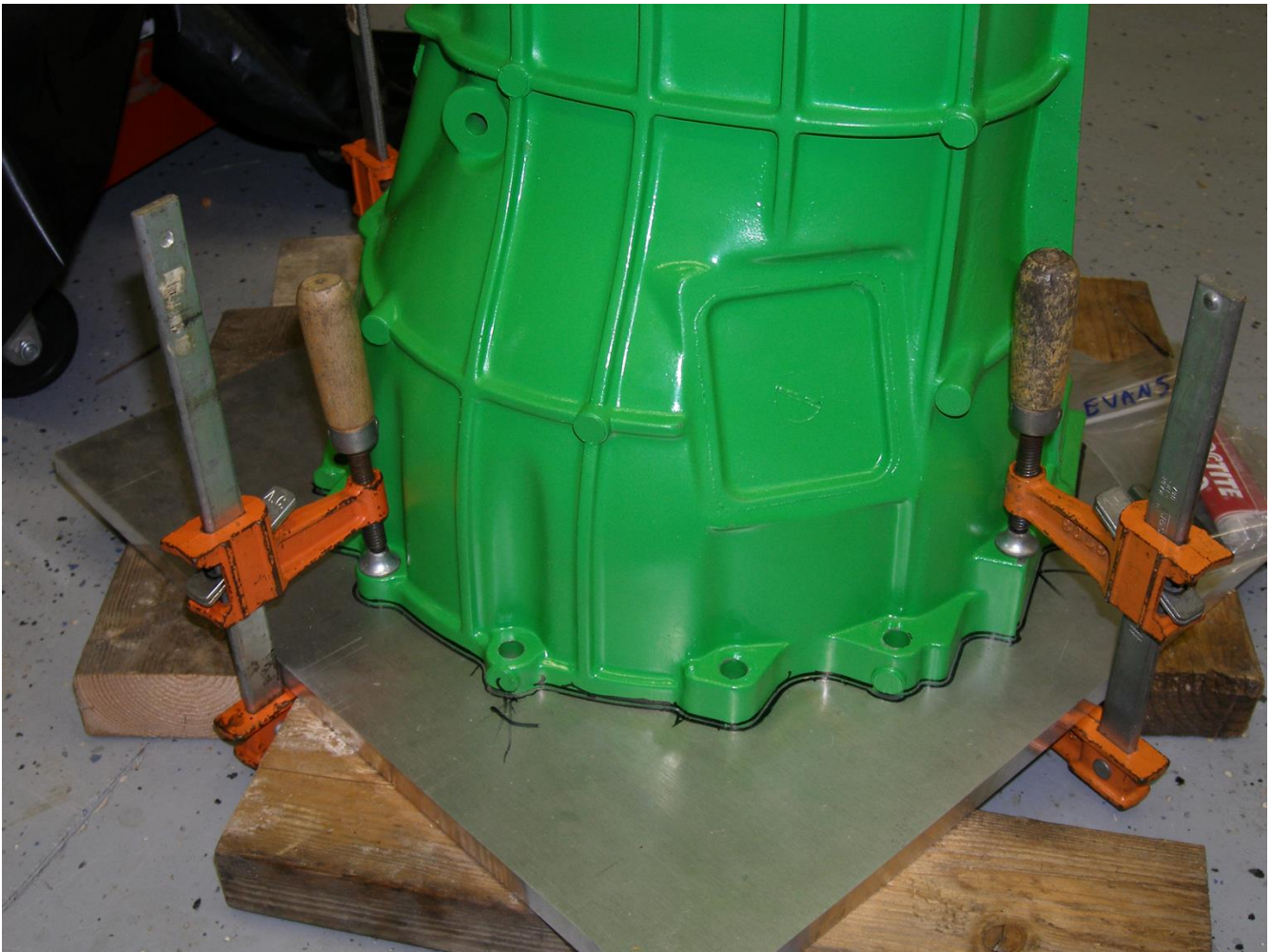
Figure 5 – 5 Detail of the 1/2” thick aluminum transmission plate securely clamped to the clutch housing face.
