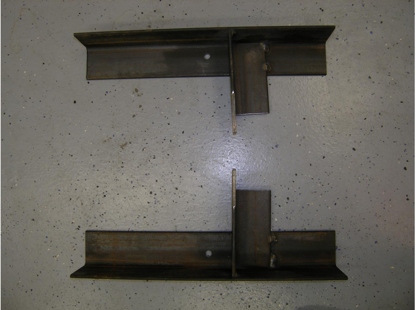
Figure 6 – 2 The motor mount parts. The long base plate (2 each), and the shorter arms (2 each)
