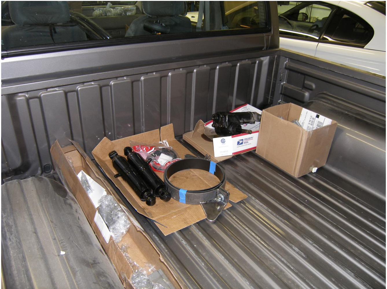
Figure 5 – 10 EV parts. The air shocks, left, and the round Motor Mount Assembly (with tape)
