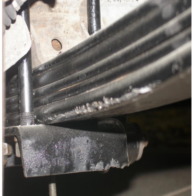
Figure 2 – 4 New “U” bolt and support piece.
