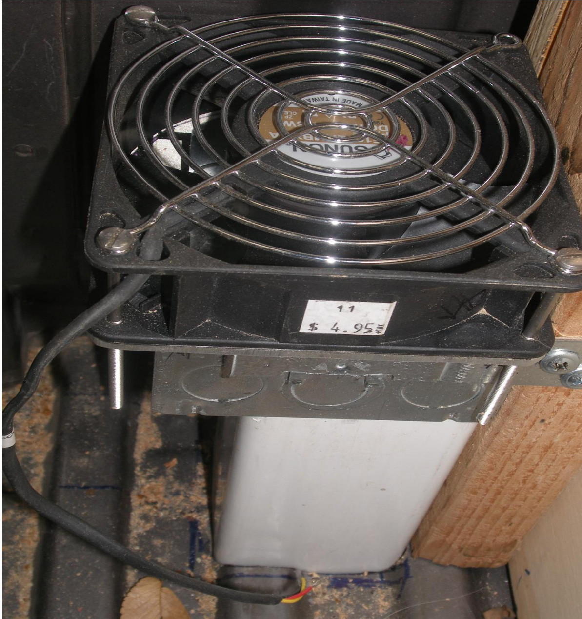
Figure 11 - 5 Installation of a 4 " brushless fan with grill attached.
