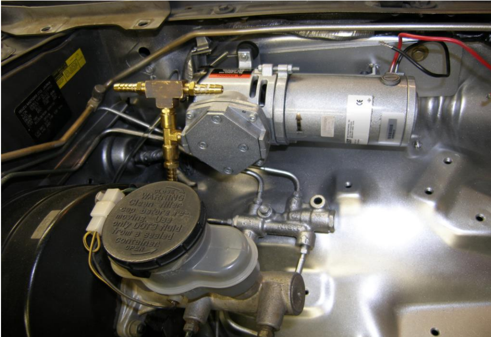
Figure 9 – 12 The Vacuum Pump with assembled brass vacuum parts ready for the rubber vacuum lines to be connected.
