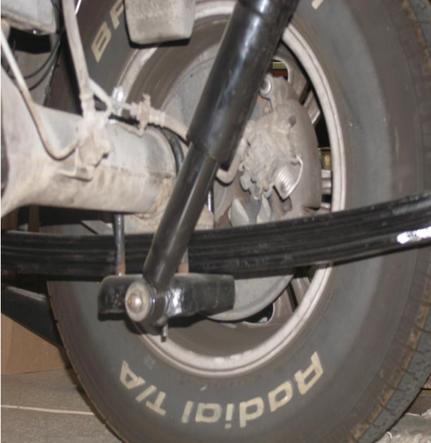
Figure 2 – 3 New leaf springs and air shocks.
