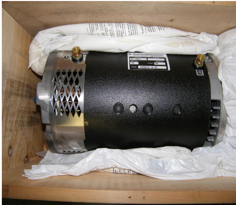
Figure 4 – 5 The electric motor in the delivery crate (170 lb.).
