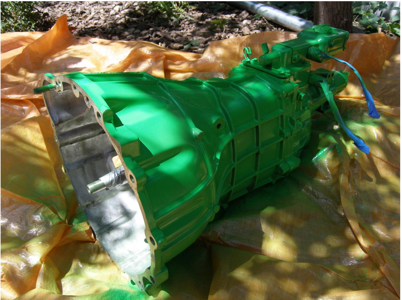
Figure 5 – 2 The stock Isuzu transmission and clutch housing showing the protruding transmission shaft.
