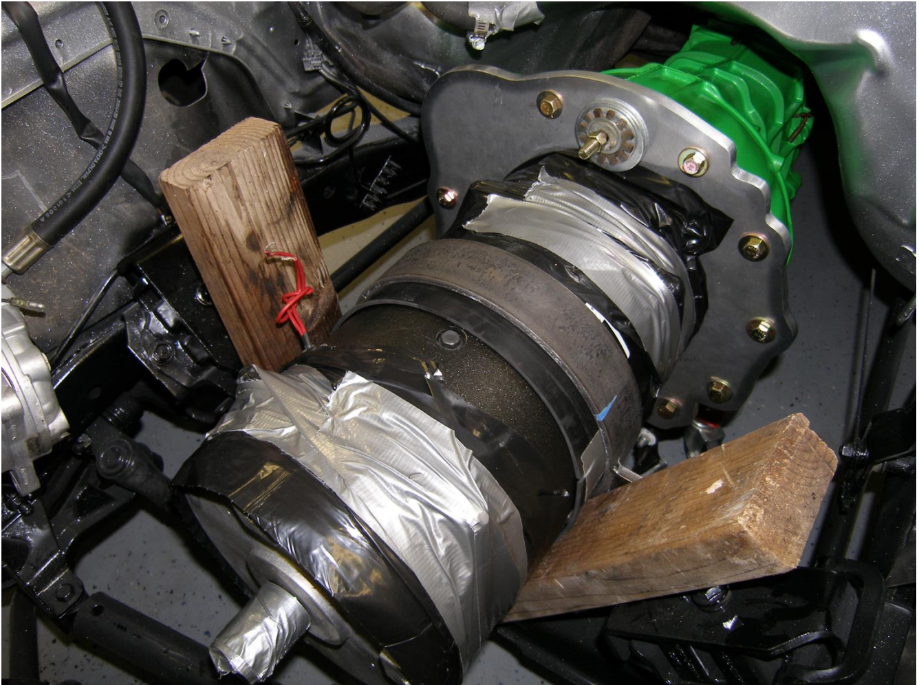
Figure 5 – 11 Stabilizing the motor in a central position.
