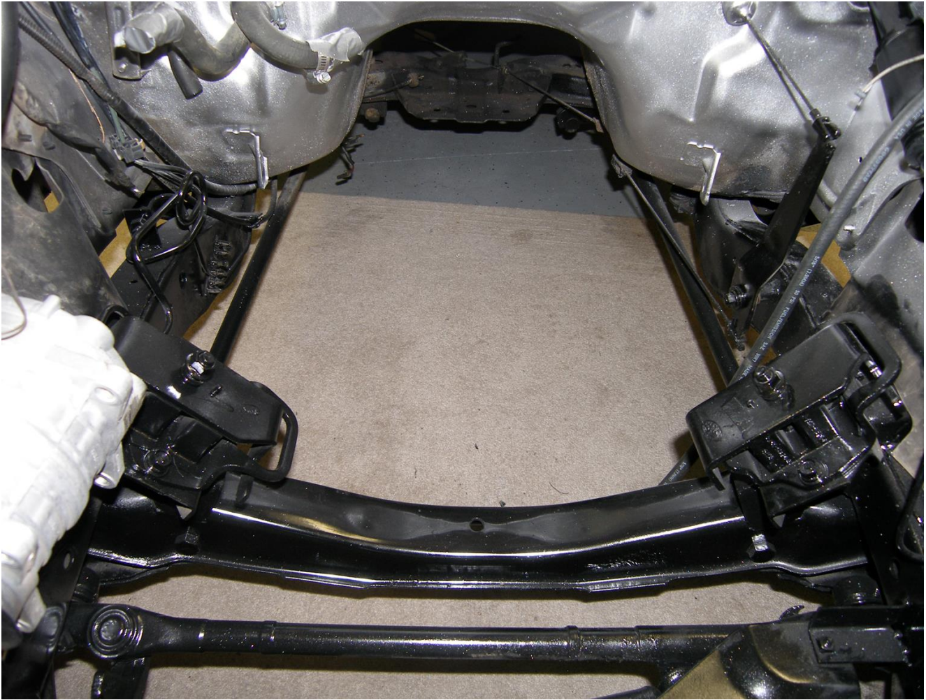
Figure 5 – 9 The motor bay ready for the placement of the electric motor (minus the rug).
