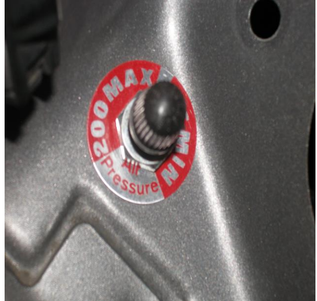
Figure 2 - 6 Air pressure valve detail.
