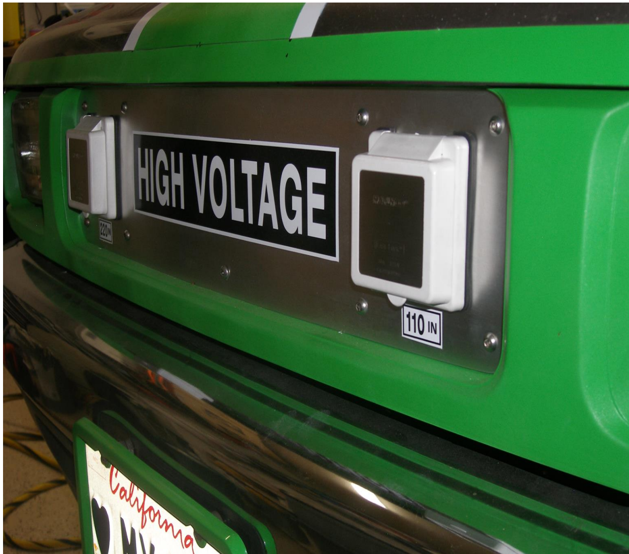
Figure 9 – 9 Mounted charging sockets
