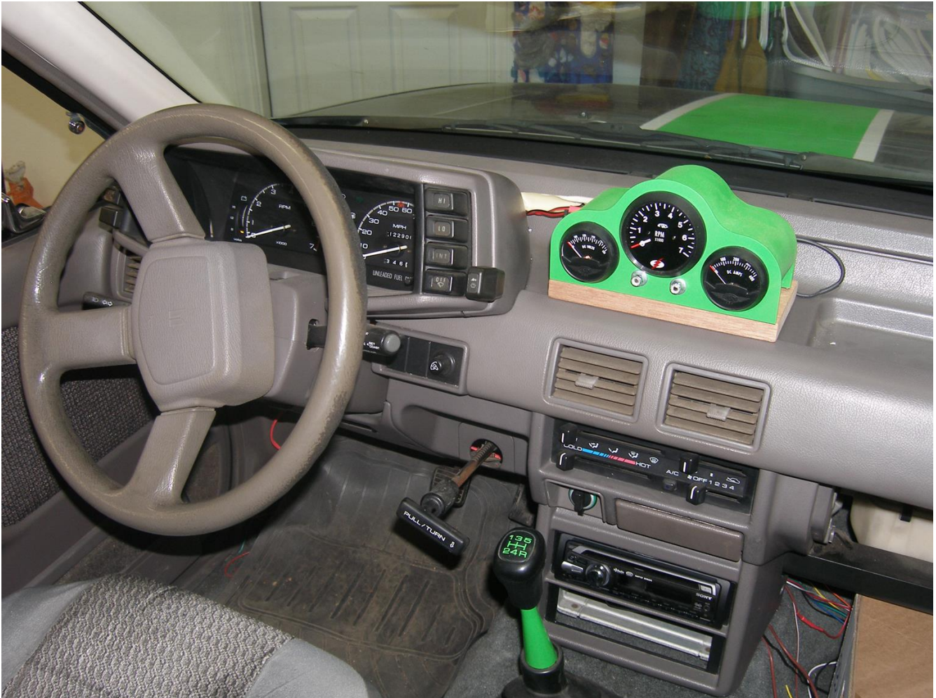
Figure 9 – 14 The stock Isuzu dashboard and instrument panel with the addition of the green EV instrument “Cluster” and the green gear shift lever and knob.
