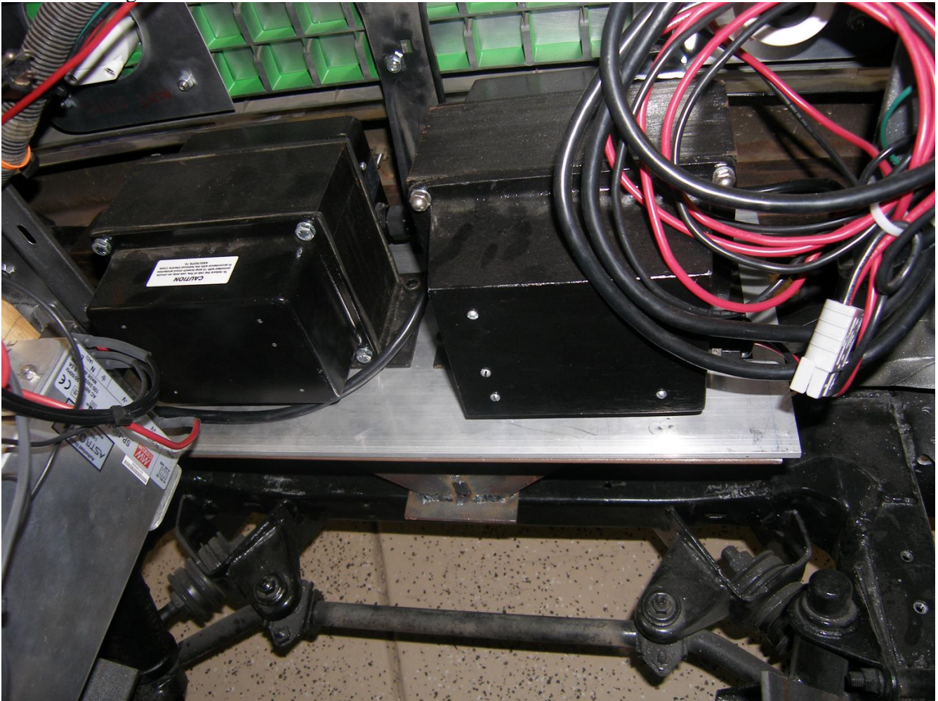
Figure 9 – 8 The 110 volt charger, shown left, 220 volt right.
