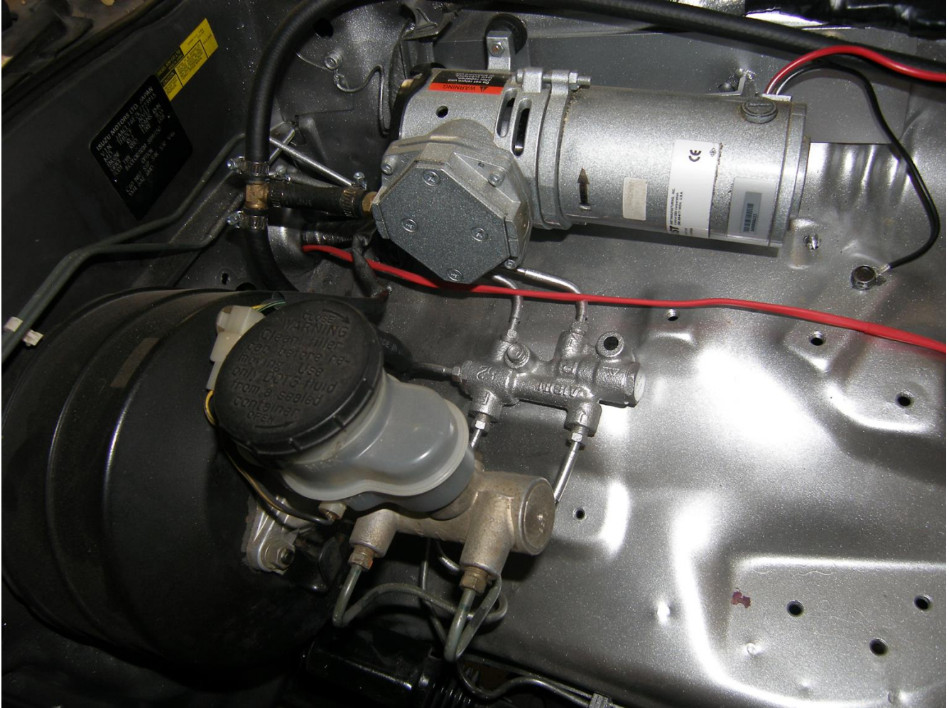
Figure 9 – 13 Vacuum Pump with fully connected EV braking system.
