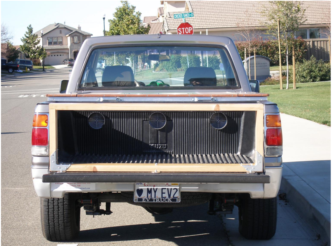
Figure 11 – 11 All three fans in place with tailgate down.
