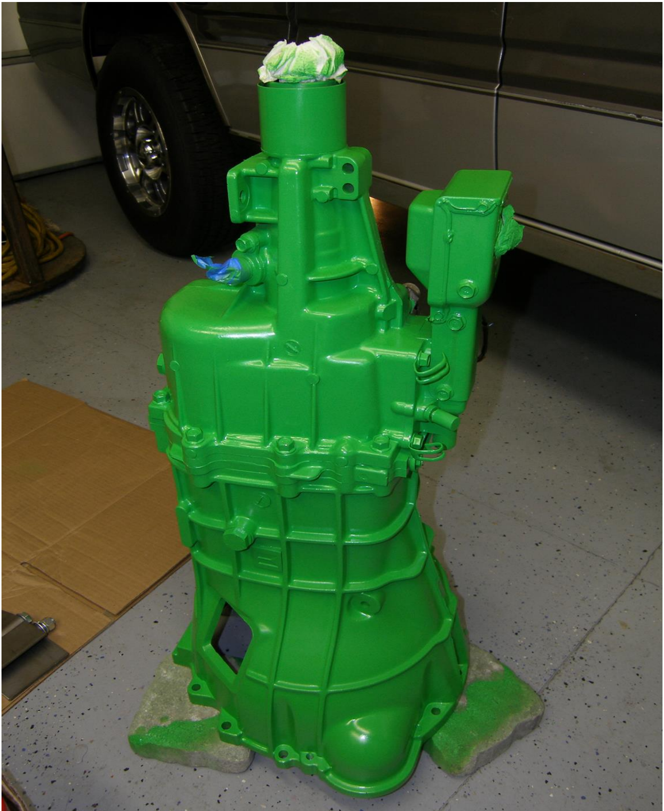
Figure 5 – 3 The newly refurbished EV transmission.
