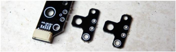
Using an M2 nut and bolt, attach 1x spacer. This makes sure that the holes line up.
