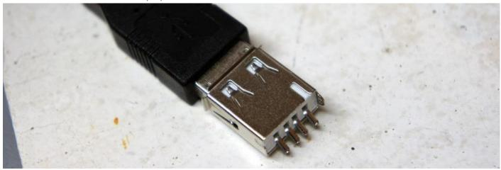
The image above shows the correct way up for the USB port. Note that there is a white square in the bottom right corner of the metal connector. THIS SQUARE MUST FACE UP (to the sky) when mounted to the back board.
