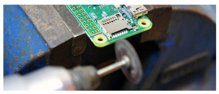
The above image shows where to cut. The YELLOW area of the PCB is the only bit that needs cutting out.
