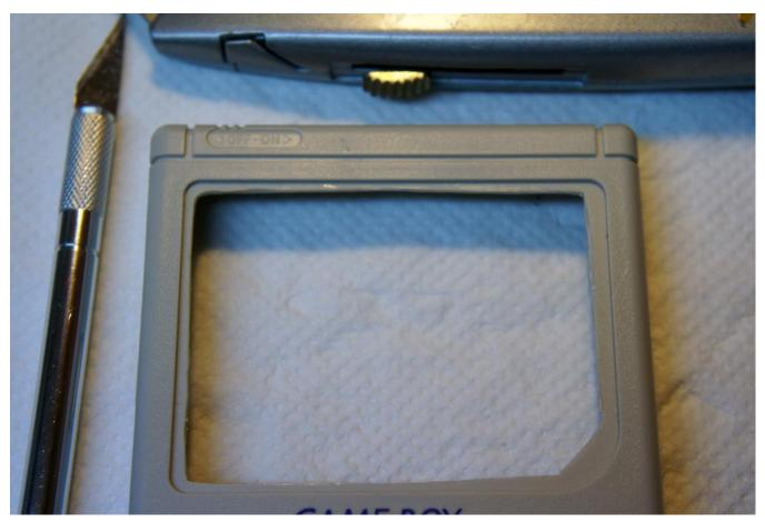
Test fit the screen overlay and see what needs to be further worked on. In the image below the right hand side and the bottom right corner need more work.
