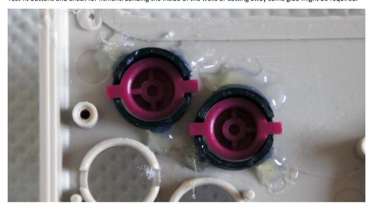
Test fit the membrane too, it will require some trimming (scissors of a knife work fine).
