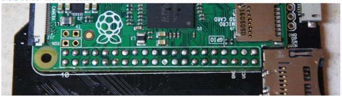
With the same technique earlier in the guide, solder the remaining pins. Use lots of flux and do each one slowly and carefully. Start from the RIGHT side and work your way left. If you have a hot air reflow station (or hot air gun) you might find it easier to 'pre-heat' the boards slightly. Any way to increase the temperature of the boards while soldering will help.
