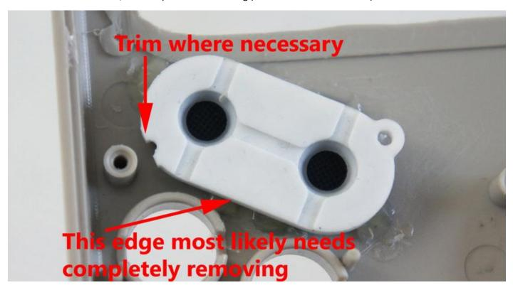
Ensure the glue doesn't interfere with the membranes. If the buttons feel a bit mushy, you may need to trim more from the membrane. A bit of trial and error and it is possible to get them to feel the same as the originals. I found that the bottom edge/lip of the membrane needed removing completely.
