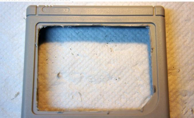
After removing the melted bits it should look like the image above.
