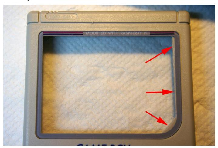
When it has been trimmed to the right size, leave it like this. DO NOT GLUE/STICK THE OVERLAY IN YET. This will be the VERY LAST thing that is fitted in this project, to avoid scratches and avoid dust on the inside of it, so for now put it somewhere safe.
