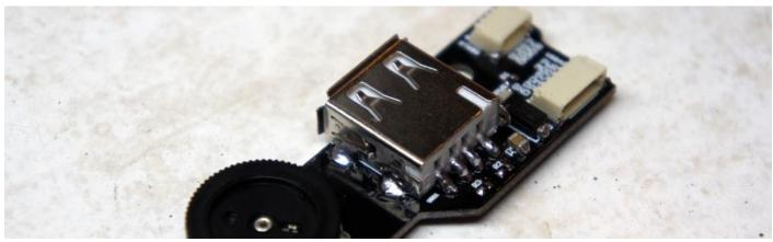
When you are 100% happy with placement, solder the remaining 4 connectors on the back. Then solder the 4 large 'support' holes (these will be a bit harder to do, make sure to hold the iron on the connectors for a while (they will be very hot and will hold their heat!)).
