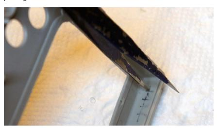
The image below shows that after pushing through, a small mark is seen on the other side. Using the needle again, push it from this side and the hole will join up.
