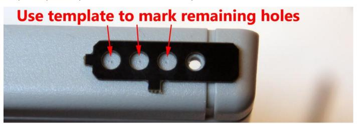
The end result should look like the image below. Be VERY careful when drilling the holes, you can see in the example image that the drill slipped on the second from left hole and has made a larger dent on the outside (the drill chuck hit the case) you should be able to avoid this if you are careful.
