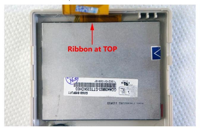
The LCD sits perfectly when mounted 1mm from the left, bottom, and right of the original mould of the DMG. The following images show what this should look like. Make sure the LCD lines up parallel to this mould line and 1mm away from all sides and it will guarantee to be in the middle and not wonky.
