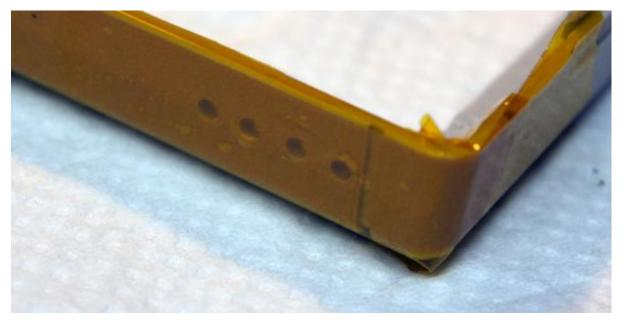
Fill each hole with hot glue. You will find that if you push glue into the holes there will be an air bubble. While the glue is hot use a needle to pop the air bubble and apply more glue. When filled, use the nozzle of the glue gun to melt the glue blobs flat. Using a knife you can trim the glue further. The image below shows the end result.
