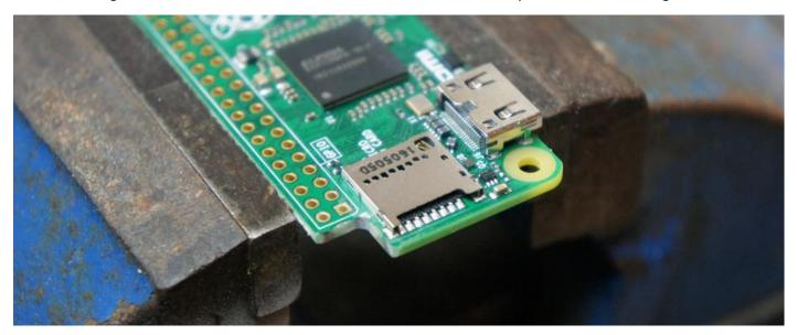
Once cut, use a file and sandpaper to smooth down and neaten up. The end result should look like the above picture. Note that there are no traces or circuitry underneath the cut out area. Just be careful of the SD card connector.
