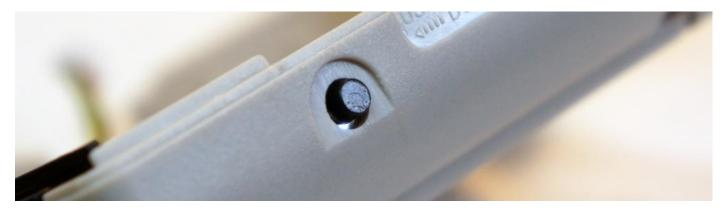
When in place, fill with glue. Using a pair of needle nose tweezers you can hold the switch from behind to make sure it lines up nicely.
