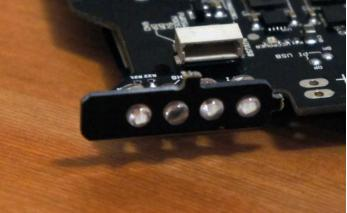
The images above show a recommended way of placing and holding the LEDs. Make to bend as close as possible to the LED base while still allowing for the LED to be parallel to the board. The legs of the LED are protruding on the side that the Pi is mounted on. It is possible to test fit the board in this state before soldering to test for fit. The entire board must slide into the case. See the following images pinout:
