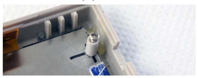
Now place the back half of case over the front. Looking down the screw holes you should be able to see the screw head perfectly. If it is not in the centre then break it off and try again (you may have to work out an angle to place the standoff down at, as the base may not be flat). If successful it should look like the image below.
