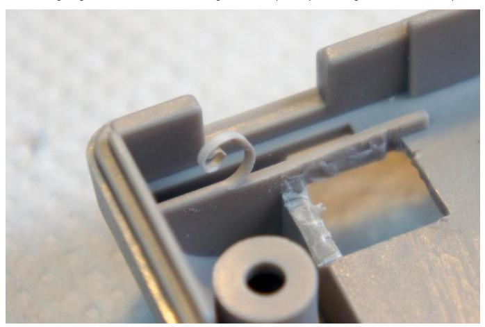
The back side should look like the following image. Neaten up with a knife if necessary. I didn't here because I am gluing the cartridge in.
