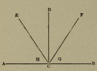
Let A B represent a polished surface, then the perpendicular ray D C falling upon this surface will be thrown directly back from C to D.
