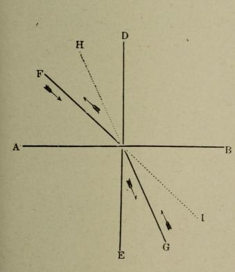
(a.) Let A B represent a surface of water, then the perpendicular ray D C will pass to D E.
