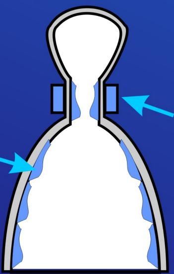
The expelled gasses have a vortex induced by a high-RPM spinning vanes motor (impeller-like) powered by a linear induction system which spins the expelled gasses through the constricting throat for stabilization purposes.
