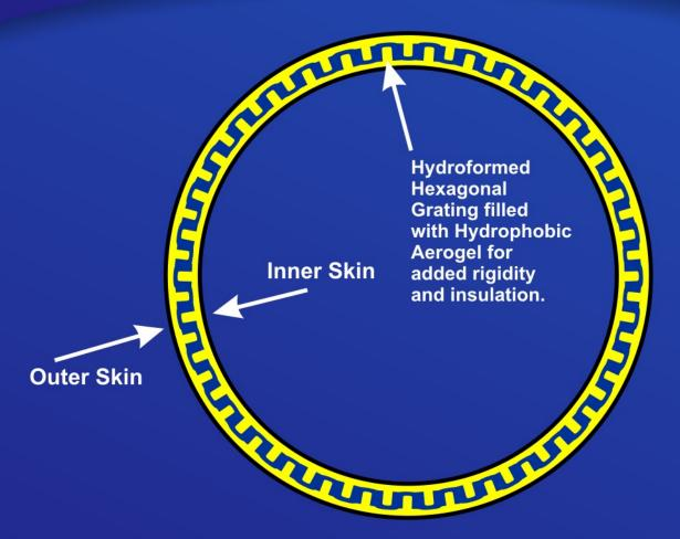
Final Result is rigid inner hexagonal grating structure containing Hydrophobic Carbon or Other Aerogel for extreme light weight and heat/cold insulation rating. Grating is covered with 1/16" or 3/32" Sheet thick film Ceramic-coated Aluminum for further rigidity.
