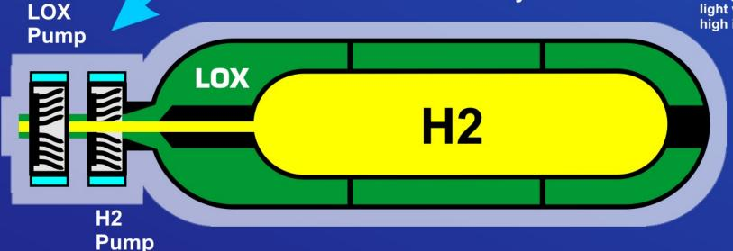
Twin Spiral Vortex Shaped Impellers have high feed rate and are linear-induction powered for high-speed and space-rated reliability.
